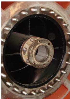
Middle part of the pump bearing
