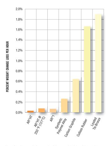
Note: Bearings made from each of the materials (size: 2 in. x 1.5 in. x 1.5 in./ 5.1 cm x 3.8 cm x 3.8 cm) were tested at 900 rpm under 25 psi (0.17 MPa). The run time of the test was eight hours. The test was conducted on 300 series SS shaft, in 95 percent water and five percent silica sand. All materials were tested at 70°F (20°C). Additionally, AR®HT was tested at 250°F (120°C) in ethylene glycol.
