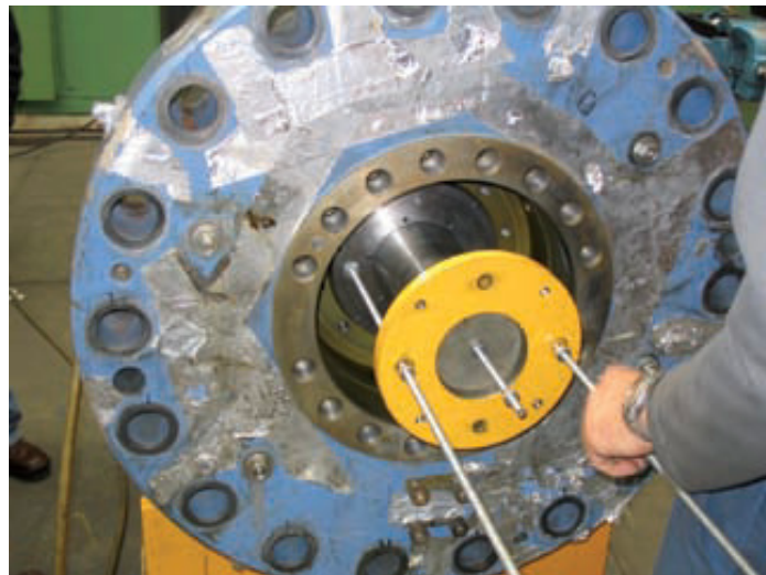
Mechanical seal removal
