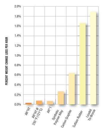
Note: Bearings made from each of the materials (size: 2 in. x 1.5 in. x 1.5 in./5.10 cm x 3.80 cm x 3.80 cm) were tested at 900 rpm under 25 psi (0.172 MPa). The run time of the test was eight hours. The test was conducted on 300 series SS shaft, in 95 percent water and 5 percent silica sand. All materials were tested at 70°F (20°C). Additionally, AR®HT was tested at 250°F (120°C) in ethylene glycol.
