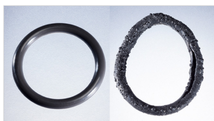
Prior best-in-class solution: before/after one week in 600°F steam
