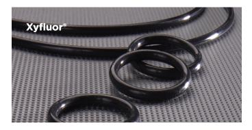
**Xyfluor**\* is a highly fluorinated compound with broad chemical resistance approaching that of FFKM and exceptional low-temperature capabilities (-76°F to 450°F/-60°C to 232°C). Xyfluor\* products include o-rings, gaskets, and custom components required for mechanical seals, metering pumps, valves, and other high-performance equipment.
