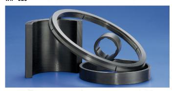
Greene, Tweed's WR® 525 is made of PEEK reinforced with continuous hoop-wound carbon fibers and is ideal for use as impeller wear rings, bushings, and case wear rings in high-pressure and high-temperature (HPHT) conditions. WR® 525's temperature range of subzero to 525°F (274°C) is suitable for stationary and rotating applications and allows users to increase efficiency with tighter wear ring clearances and decrease potential damage.
