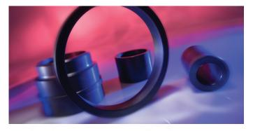
Greene, Tweed's WR® 300 is composed of PEEK reinforced with short, random carbon fibers with a temperature range from subzero to 275°F (135°C). WR® 300 is suitable for general wear resistance applications and is often used in pump bushings and cases or impeller wear rings.
