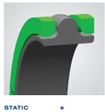
A double-acting rod or piston seal with an outstanding combination of easy installation, low leakage and long service life for exceptional performance in many static and dynamic sealing applications. The G-T ring offers better extrusion resistance and eliminates spiral failure when compared to an O-ring and Back-up ring assembly. Click to learn more.
