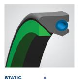
The CSA seal consists of an elastomer jacket, for outstanding sealing, energized by a coil spring. The coil spring overcomes sealing problems caused by high application ovality, excessive side forces, or high temperature compression set. Click to learn more.
