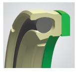
A unidirectional, "self-venting" seal design consisting of a PTFE jacket and an elastomer O-ring energizer. The seal design and energizer allow installation into "closed-groove" configurations for most sizes. The seal can also be complemented with a high modulus backup ring for higher pressures or larger sealing gaps. Along with the "self-venting" capability, the ESE design offers low operating friction along a wide operational temperature range. Click to learn more.
