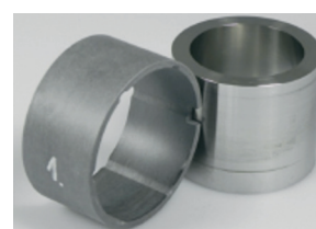
Journal bearing #1 after third test (105-minute test duration)
