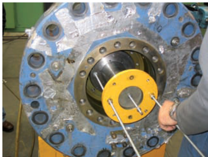
Mechanical seal removal
