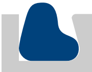
Glandlock® Seal (Half Dovetail Gland)
