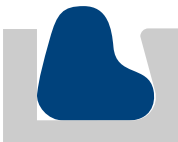
Glandlock® Seal (Half Dovetail Gland)
