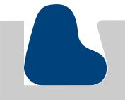
Glandlock® Seal (Half Dovetail Gland)
