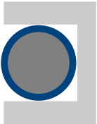
Plastic Encapsulated O-ring (All Glands)
