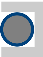
Plastic Encapsulated O-ring (All Glands)
