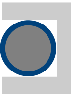
Plastic Encapsulated O-ring (All Glands)
