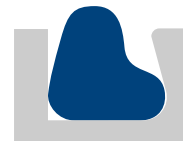
Glandlock® Seal (Half Dovetail Gland)
