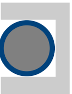
Plastic Encapsulated O-ring (All Glands)
