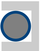
Plastic Encapsulated O-ring (All Glands)
